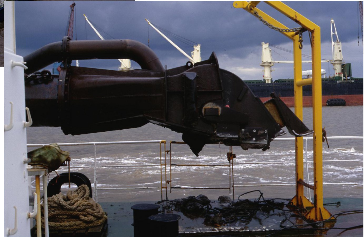
Trailing suction hopper dredger
